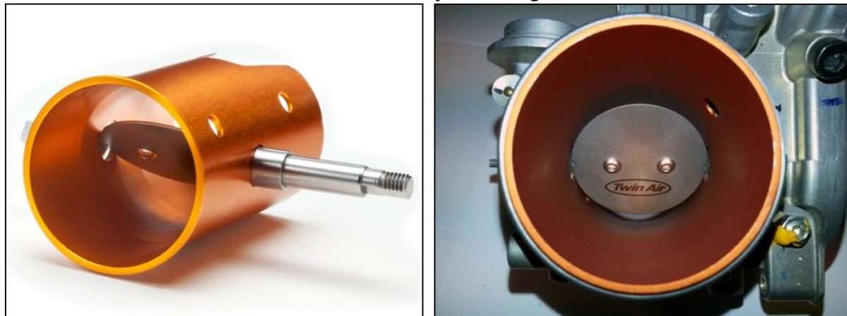
The Powerflow Throttle Body Kit **Configuration #2** is designed for increasing top end power gains by reducing the surface area of the throttle body valve. This configuration does not use the orange intake tube.
